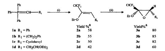
(i) CICF<sub>2</sub>CO<sub>2</sub>Et, THF. Reflux 3 h, (ii) MCPBA, CH<sub>2</sub>Cl<sub>2</sub>, R T 48 h.
